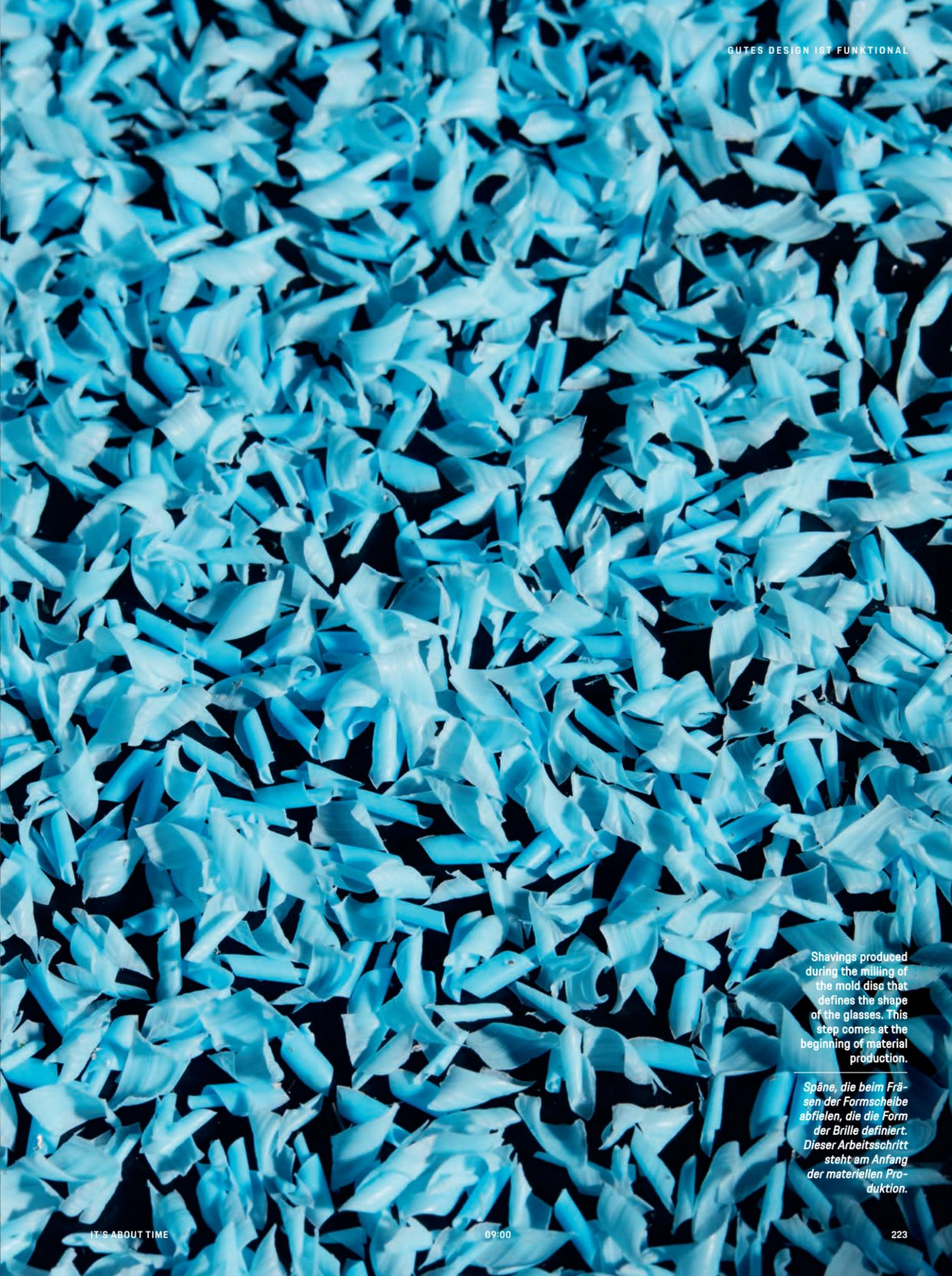
Shavings produced during the milling of the mold disc that defines the shape of the glasses. This step comes at the beginning of material production.
