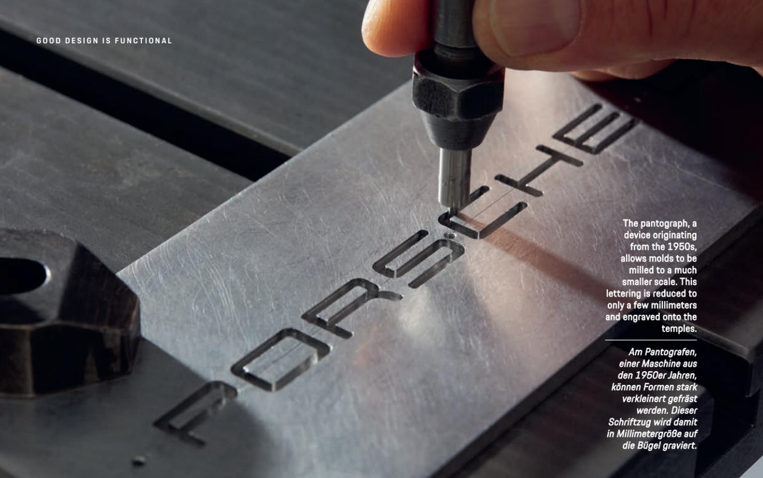
The pantograph, a device originating from the 1950s, allows molds to be milled to a much smaller scale. This lettering is reduced to only a few millimeters and engraved onto the temples.
