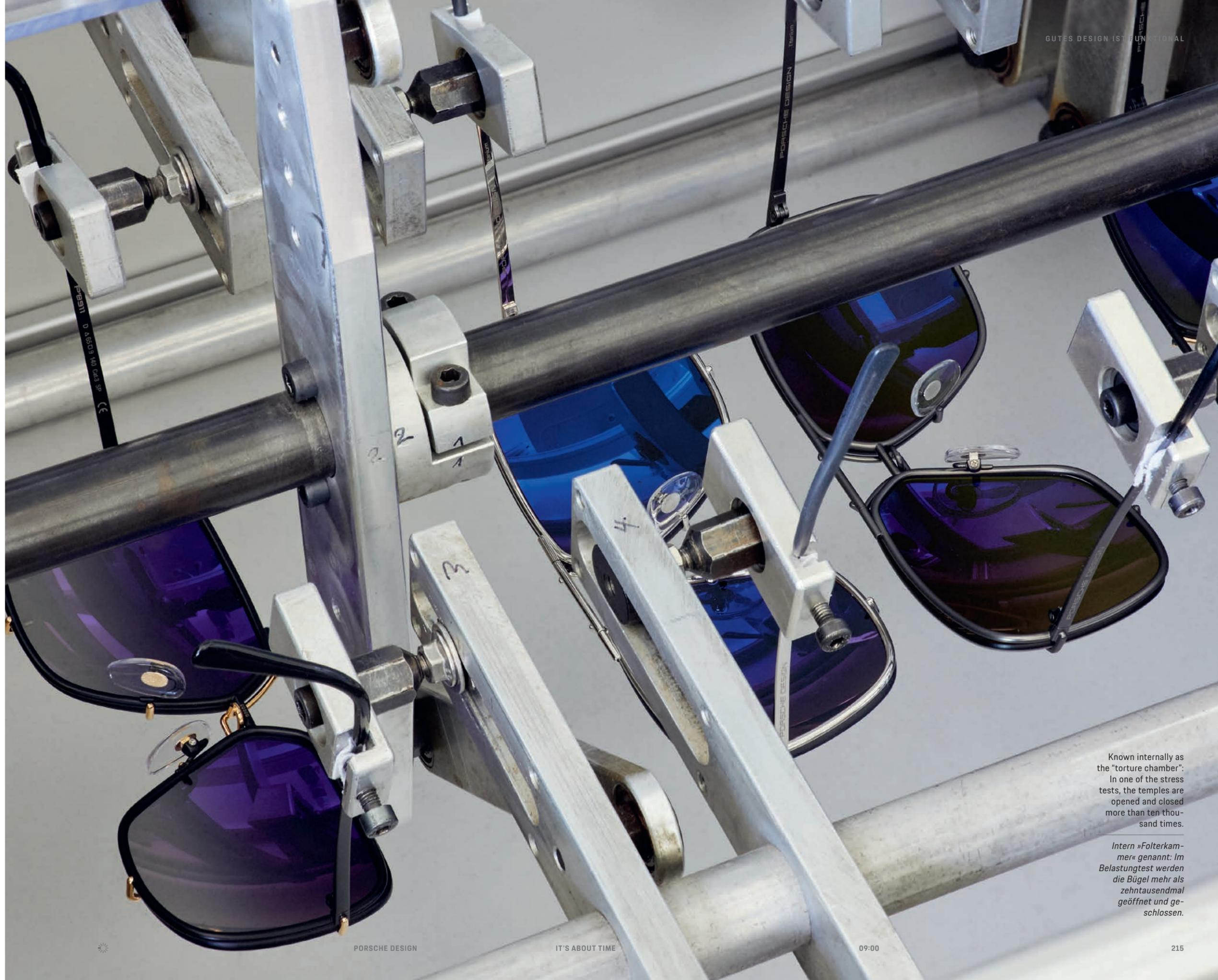
Known internally as the “torture chamber”: In one of the stress tests, the temples are opened and closed more than ten thousand times.
